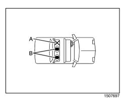
A. Occupant prohibited B. Child restraint using LATCH
